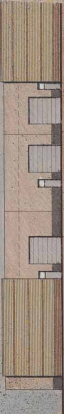
rear elevation study scale: 1/16"=1'-0" tilt concrete walls, banded masonry walls in earth tones with aluminum color roll up and access doors.
