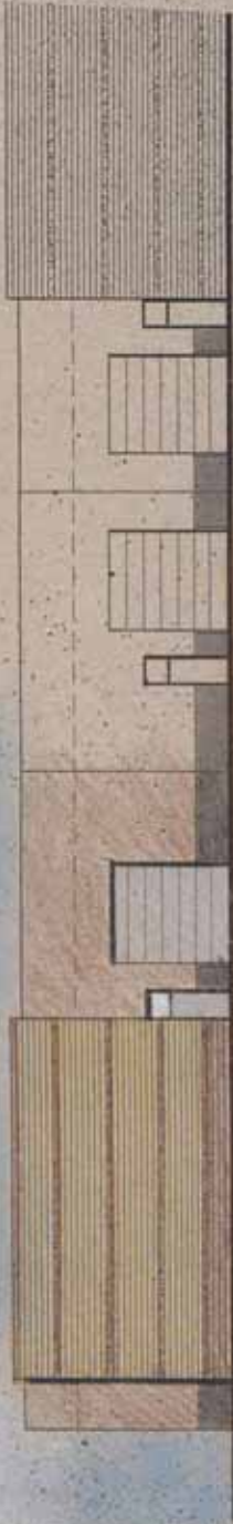
rear elevation study scale: 1/16"=1'-0" fill concrete walls, banded masonry walls in earth tones with aluminum color roll up and access doors
