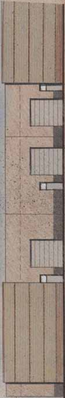
rear elevation study scale: 1/16"=1'-0" tilt concrete walls, banded masonry walls in earth tones with aluminum color roll up and access doors
